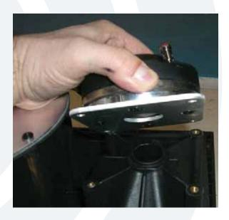
The high frequency driver should easily lift right off of the horn assembly. Holding down the horn assembly with one hand while lifting up on the driver with the other hand may help.
